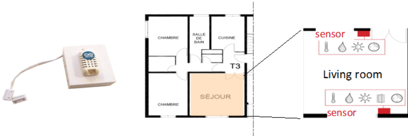
Sensors placed inside a flat
